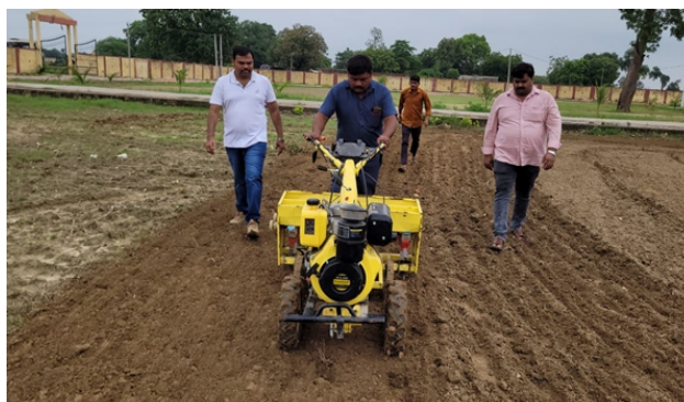
FLD on direct seeded rice through manually power operated seed drill machine at KVK Sultanpur II
